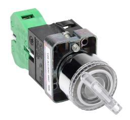
AutomationDirect selector switch, 22mm, 2-position, spring return from right, incandescent illuminated, (1) N.O. contact(s), metal base, metal bezel, Operator: clear, knob, 30mm, round, plastic, 120 VAC/VDC, full voltage.
