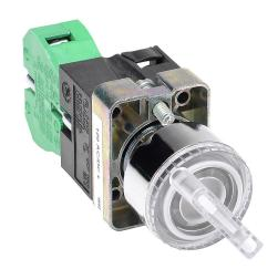
AutomationDirect selector switch, 22mm, 2-position, spring return from right, LED illuminated, (1) N.O. contact(s), metal base, metal bezel, Operator: clear, knob, 30mm, round, plastic, 120 VAC/VDC, full voltage.
