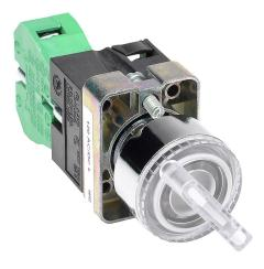
AutomationDirect selector switch, 22mm, 2-position, spring return from right, LED illuminated, (1) N.O. contact(s), metal base, metal bezel, Operator: clear, knob, 30mm, round, plastic, 120 VAC/ VDC, full voltage.
