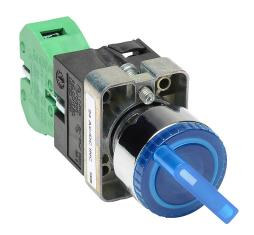
AutomationDirect selector switch, 22mm, 2-position, spring return from right, incandescent illuminated, (1) N.O. contact(s), metal base, metal bezel, Operator: blue, knob, 30mm, round, plastic, 24 VAC/VDC, full voltage.
