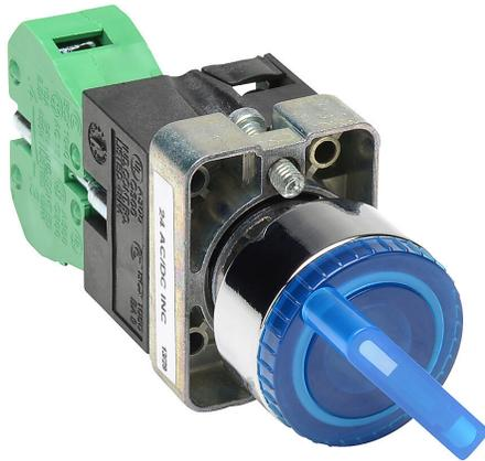
AutomationDirect selector switch, 22mm, 2-position, spring return from right, incandescent illuminated, (1) N.O. contact(s), metal base, metal bezel, Operator: blue, knob, 30mm, round, plastic, 24 VAC/VDC, full voltage.
