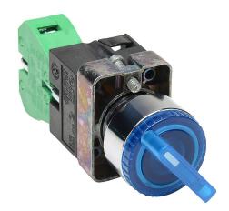
AutomationDirect selector switch, 22mm, 2-position, spring return from right, LED illuminated, (1) N.O. contact(s), metal base, metal bezel, Operator: blue, knob, 30mm, round, plastic, 120 VAC/VDC, full voltage.
