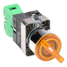
AutomationDirect selector switch, 22mm, 2-position, spring return from right, incandescent illuminated, (1) N.O. contact(s), metal base, metal bezel, Operator: yellow, knob, 30mm, round, plastic, 24 VAC/VDC, full voltage.
