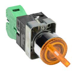
AutomationDirect selector switch, 22mm, 2-position, spring return from right, LED illuminated, (1) N.O. contact(s), metal base, metal bezel, Operator: yellow, knob, 30mm, round, plastic, 24 VAC/VDC, full voltage.
