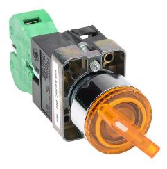
AutomationDirect selector switch, 22mm, 2-position, spring return from right, incandescent illuminated, (1) N.O. contact(s), metal base, metal bezel, Operator: yellow, knob, 30mm, round, plastic, 120 VAC/VDC, full voltage.
