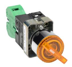
AutomationDirect selector switch, 22mm, 2-position, spring return from right, LED illuminated, (1) N.O. contact(s), metal base, metal bezel, Operator: yellow, knob, 30mm, round, plastic, 120 VAC/VDC, full voltage.
