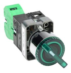
AutomationDirect selector switch, 22mm, 2-position, spring return from right, incandescent illuminated, (1) N.O. contact(s), metal base, metal bezel, Operator: green, knob, 30mm, round, plastic, 24 VAC/VDC, full voltage.
