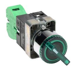
AutomationDirect selector switch, 22mm, 2-position, spring return from right, LED illuminated, (1) N.O. contact(s), metal base, metal bezel, Operator: green, knob, 30mm, round, plastic, 24 VAC/VDC, full voltage.
