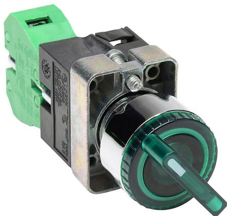
AutomationDirect selector switch, 22mm, 2-position, spring return from right, LED illuminated, (1) N.O. contact(s), metal base, metal bezel, Operator: green, knob, 30mm, round, plastic, 24 VAC/VDC, full voltage.
