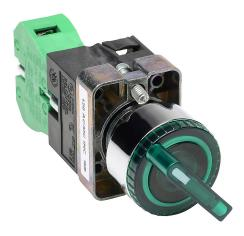
AutomationDirect selector switch, 22mm, 2-position, spring return from right, incandescent illuminated, (1) N.O. contact(s), metal base, metal bezel, Operator: green, knob, 30mm, round, plastic, 120 VAC/VDC, full voltage.
