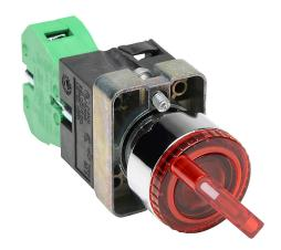
AutomationDirect selector switch, 22mm, 2-position, spring return from right, incandescent illuminated, (1) N.O. contact(s), metal base, metal bezel, Operator: red, knob, 30mm, round, plastic, 24 VAC/VDC, full voltage.
