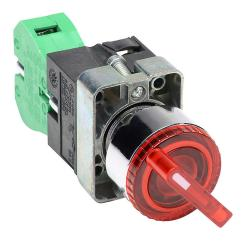
AutomationDirect selector switch, 22mm, 2-position, spring return from right, LED illuminated, (1) N.O. contact(s), metal base, metal bezel, Operator: red, knob, 30mm, round, plastic, 24 VAC/ VDC, full voltage.
