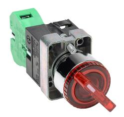
AutomationDirect selector switch, 22mm, 2-position, spring return from right, incandescent illuminated, (1) N.O. contact(s), metal base, metal bezel, Operator: red, knob, 30mm, round, plastic, 120 VAC/VDC, full voltage.
