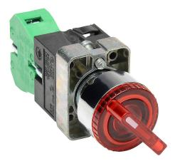
AutomationDirect selector switch, 22mm, 2-position, spring return from right, LED illuminated, (1) N.O. contact(s), metal base, metal bezel, Operator: red, knob, 30mm, round, plastic, 120 VAC/ VDC, full voltage.
