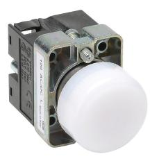
AutomationDirect LED indicating light, permanent light function, IP65, 22mm, white, 30mm, round, metal base, 120 VAC/VDC, full voltage.
