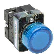
AutomationDirect LED indicating light, permanent light function, IP65, 22mm, blue, 30mm, round, metal base, 24 VAC/VDC, full voltage.
