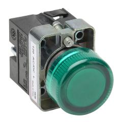
AutomationDirect LED indicating light, permanent light function, IP65, 22mm, green, 30mm, round, metal base, 120 VAC/VDC, full voltage.
