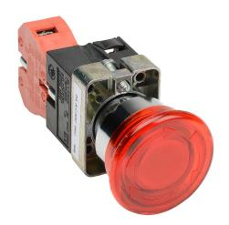
AutomationDirect pushbutton, IP65, 22mm, twist-to-release, incandescent illuminated, (1) N.C. contact(s), metal base, metal bezel, Operator: red, mushroom, 40mm, round, plastic, 24 VAC/VDC, full voltage.
