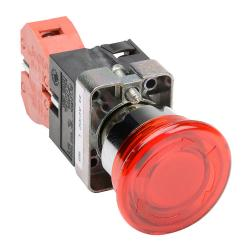
AutomationDirect pushbutton, IP65, 22mm, twist-to-release, LED illuminated, (1) N.C. contact(s), metal base, metal bezel, Operator: red, mushroom, 40mm, round, plastic, 24 VAC/VDC, full voltage.
