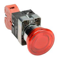
AutomationDirect pushbutton, IP65, 22mm, twist-to-release, LED illuminated, (1) N.C. contact(s), metal base, metal bezel, Operator: red, mushroom, 40mm, round, plastic, 120 VAC/VDC, full voltage.
