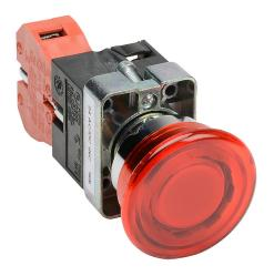
AutomationDirect pushbutton, IP65, 22mm, momentary, incandescent illuminated, (1) N.C. contact(s), metal base, metal bezel, Operator: red, mushroom, 40mm, round, plastic, 24 VAC/VDC, full voltage.
