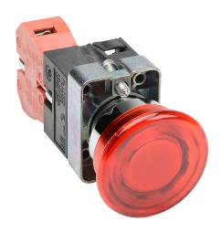
AutomationDirect pushbutton, IP65, 22mm, momentary, LED illuminated, (1) N.C. contact(s), metal base, metal bezel, Operator: red, mushroom, 40mm, round, plastic, 24 VAC/VDC, full voltage.
