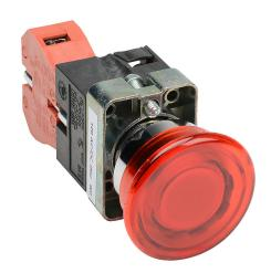
AutomationDirect pushbutton, IP65, 22mm, momentary, incandescent illuminated, (1) N.C. contact(s), metal base, metal bezel, Operator: red, mushroom, 40mm, round, plastic, 120 VAC/VDC, full voltage.
