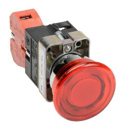
AutomationDirect pushbutton, IP65, 22mm, momentary, LED illuminated, (1) N.C. contact(s), metal base, metal bezel, Operator: red, mushroom, 40mm, round, plastic, 120 VAC/VDC, full voltage.
