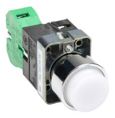
AutomationDirect pushbutton, IP65, 22mm, momentary, incandescent illuminated, (1) N.O. contact(s), metal base, metal bezel, Operator: white, extended, 30mm, round, plastic, 24 VAC/VDC, full voltage.
