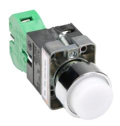
AutomationDirect pushbutton, IP65, 22mm, momentary, incandescent illuminated, (1) N.O. contact(s), metal base, metal bezel, Operator: white, extended, 30mm, round, plastic, 120 VAC/VDC, full voltage.
