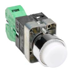
AutomationDirect pushbutton, IP65, 22mm, momentary, LED illuminated, (1) N.O. contact(s), metal base, metal bezel, Operator: white, extended, 30mm, round, plastic, 120 VAC/VDC, full voltage.
