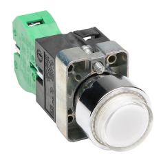
AutomationDirect pushbutton, IP65, 22mm, momentary, incandescent illuminated, (1) N.O. contact(s), metal base, metal bezel, Operator: clear, extended, 30mm, round, plastic, 24 VAC/VDC, full voltage.
