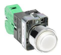
AutomationDirect pushbutton, IP65, 22mm, momentary, LED illuminated, (1) N.O. contact(s), metal base, metal bezel, Operator: clear, extended, 30mm, round, plastic, 24 VAC/VDC, full voltage.
