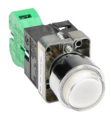
AutomationDirect pushbutton, IP65, 22mm, momentary, incandescent illuminated, (1) N.O. contact(s), metal base, metal bezel, Operator: clear, extended, 30mm, round, plastic, 120 VAC/VDC, full voltage.
