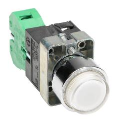
AutomationDirect pushbutton, IP65, 22mm, momentary, LED illuminated, (1) N.O. contact(s), metal base, metal bezel, Operator: clear, extended, 30mm, round, plastic, 120 VAC/VDC, full voltage.
