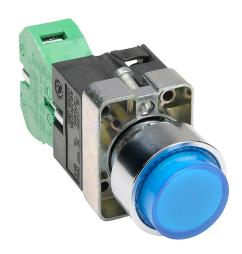
AutomationDirect pushbutton, IP65, 22mm, momentary, LED illuminated, (1) N.O. contact(s), metal base, metal bezel, Operator: blue, extended, 30mm, round, plastic, 24 VAC/VDC, full voltage.
