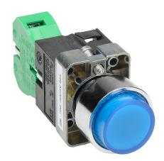
AutomationDirect pushbutton, IP65, 22mm, momentary, incandescent illuminated, (1) N.O. contact(s), metal base, metal bezel, Operator: blue, extended, 30mm, round, plastic, 120 VAC/VDC, full voltage.
