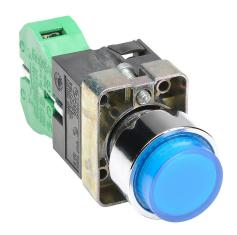
AutomationDirect pushbutton, IP65, 22mm, momentary, LED illuminated, (1) N.O. contact(s), metal base, metal bezel, Operator: blue, extended, 30mm, round, plastic, 120 VAC/VDC, full voltage.
