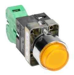
AutomationDirect pushbutton, IP65, 22mm, momentary, incandescent illuminated, (1) N.O. contact(s), metal base, metal bezel, Operator: yellow, extended, 30mm, round, plastic, 24 VAC/VDC, full voltage.
