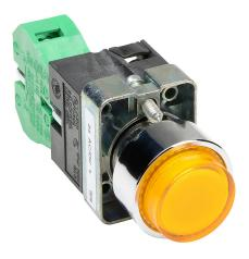
AutomationDirect pushbutton, IP65, 22mm, momentary, LED illuminated, (1) N.O. contact(s), metal base, metal bezel, Operator: yellow, extended, 30mm, round, plastic, 24 VAC/VDC, full voltage.
