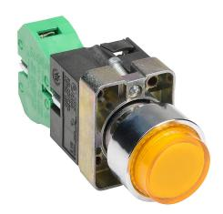
AutomationDirect pushbutton, IP65, 22mm, momentary, incandescent illuminated, (1) N.O. contact(s), metal base, metal bezel, Operator: yellow, extended, 30mm, round, plastic, 120 VAC/VDC, full voltage.
