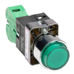
AutomationDirect pushbutton, IP65, 22mm, momentary, incandescent illuminated, (1) N.O. contact(s), metal base, metal bezel, Operator: green, extended, 30mm, round, plastic, 24 VAC/VDC, full voltage.
