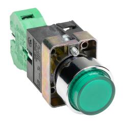
AutomationDirect pushbutton, IP65, 22mm, momentary, LED illuminated, (1) N.O. contact(s), metal base, metal bezel, Operator: green, extended, 30mm, round, plastic, 24 VAC/VDC, full voltage.
