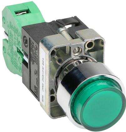
AutomationDirect pushbutton, IP65, 22mm, momentary, incandescent illuminated, (1) N.O. contact(s), metal base, metal bezel, Operator: green, extended, 30mm, round, plastic, 120 VAC/VDC, full voltage.
