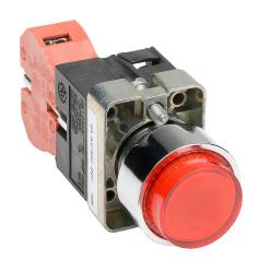
AutomationDirect pushbutton, IP65, 22mm, momentary, incandescent illuminated, (1) N.C. contact(s), metal base, metal bezel, Operator: red, extended, 30mm, round, plastic, 24 VAC/VDC, full voltage.
