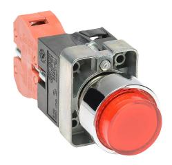
AutomationDirect pushbutton, IP65, 22mm, momentary, LED illuminated, (1) N.C. contact(s), metal base, metal bezel, Operator: red, extended, 30mm, round, plastic, 24 VAC/VDC, full voltage.
