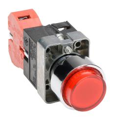
AutomationDirect pushbutton, IP65, 22mm, momentary, incandescent illuminated, (1) N.C. contact(s), metal base, metal bezel, Operator: red, extended, 30mm, round, plastic, 120 VAC/VDC, full voltage.
