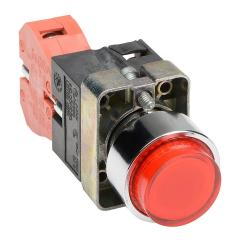
AutomationDirect pushbutton, IP65, 22mm, momentary, LED illuminated, (1) N.C. contact(s), metal base, metal bezel, Operator: red, extended, 30mm, round, plastic, 120 VAC/VDC, full voltage.
