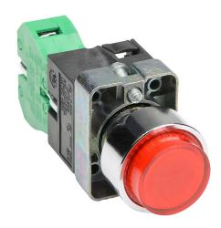
AutomationDirect pushbutton, IP65, 22mm, momentary, LED illuminated, (1) N.O. contact(s), metal base, metal bezel, Operator: red, extended, 30mm, round, plastic, 120 VAC/VDC, full voltage.
