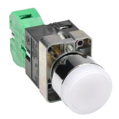
AutomationDirect pushbutton, IP65, 22mm, momentary, incandescent illuminated, (1) N.O. contact(s), metal base, metal bezel, plastic ring, Operator: white, flush, 30mm, round, plastic, 24 VAC/VDC, full voltage.
