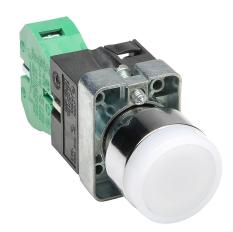
AutomationDirect pushbutton, IP65, 22mm, momentary, incandescent illuminated, (1) N.O. contact(s), metal base, metal bezel, plastic ring, Operator: white, flush, 30mm, round, plastic, 120 VAC/VDC, full voltage.
