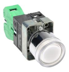
AutomationDirect pushbutton, IP65, 22mm, momentary, incandescent illuminated, (1) N.O. contact(s), metal base, metal bezel, plastic ring, Operator: clear, flush, 30mm, round, plastic, 24 VAC/VDC, full voltage.
