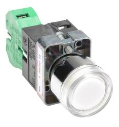
AutomationDirect pushbutton, IP65, 22mm, momentary, LED illuminated, (1) N.O. contact(s), metal base, metal bezel, plastic ring, Operator: clear, flush, 30mm, round, plastic, 24 VAC/VDC, full voltage.
